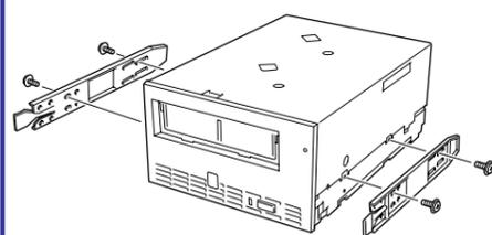
**Tips** Some servers require the rails to be used. For details on how to install the rails, refer to the server's operating manual.
