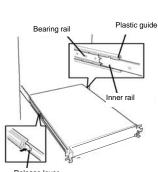
(4) Fasten the screws loosened in step 1 to fix the slide bracket.
